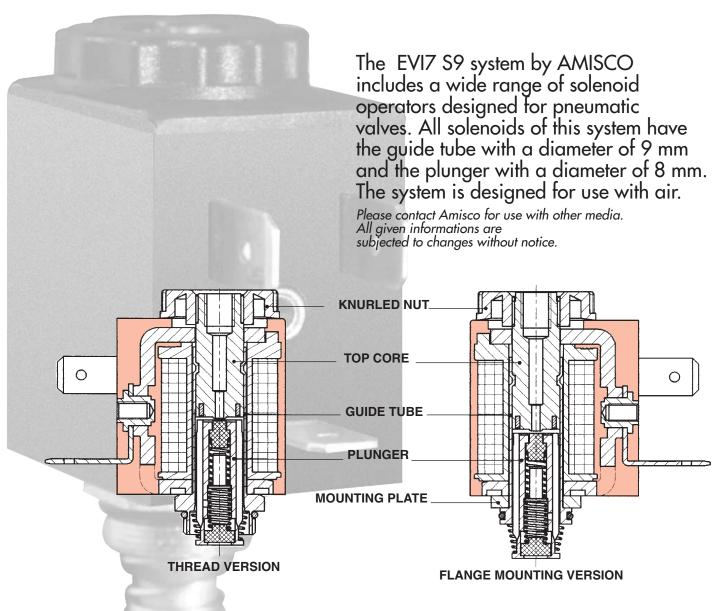
The coil is available in different sizes and with different electrical terminations. Types, power and other characteristics are described in the following pages. All coils feature:
